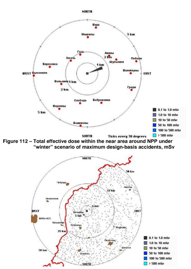
Figure 113 – Total effective dose within the remote area around NPP under «winter» scenario of maximum design-basis accidents, mSv
