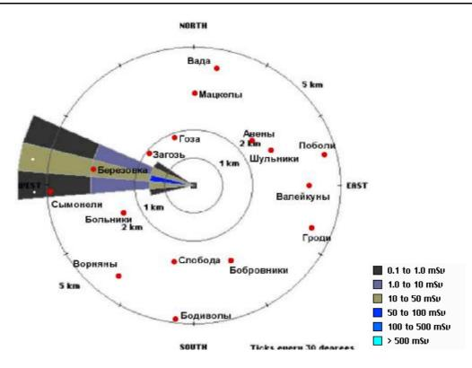
Figure 116 – Total effective dose in the area near the NPP at beyond design basis accident, mSv
