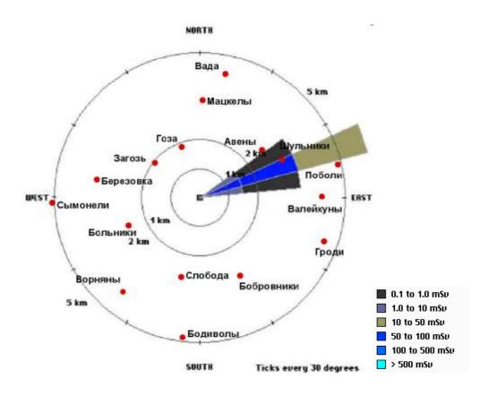
Figure 120 – Total effective dose within the area near the NPP at beyond design basis accident, mSv
