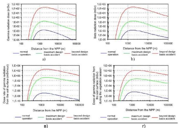
Figure 110 – Forecasted doses from external gamma radiation in gases and aerosols (a), from external beta radiation in the cloud (b), dose rates of external gamma radiation from the soil surface (c), doses of external gamma radiation from the soil surface during the vegetation period (d)
