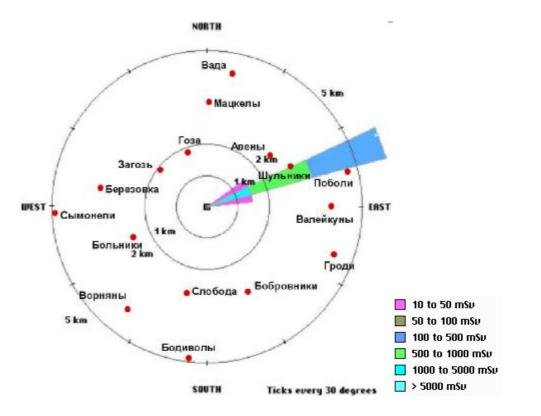
Figure 122 – Dose of irradiation over the thyroid gland within the area near the NPP at beyond design basis accident, mSv (mGy)
