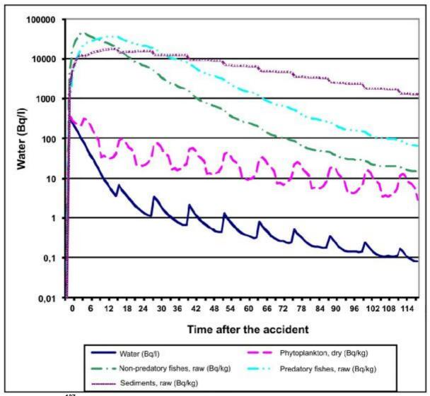
Figure 111 – <sup>137</sup>Cs content in water, bottom sediments, phytoplankton and bodies of nonpredatory and predatory fishes in case of an accident beyond the design basis
