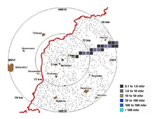
Figure 121 – Total effective dose within the area remote from the NPP at beyond design basis accident, mSv
