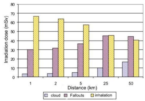
Figure 125 – Contribution of various components of irradiation doses in the total dose versus distance from the source of emission
