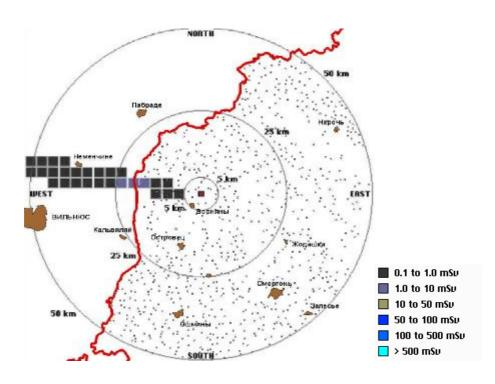
Figure 117 – Total effective dose in the area remoted from the NPP at beyond design basis accident, mSv
