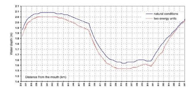
Figure 88 – The results of forecast for changes of the level mode (the stream depth) in the river Viliya in case of water supply facility construction, for water flow rates near the minimum average daily quantities during the summer and autumn low water level period (97 % exceedance probability)
