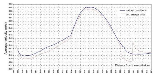
Figure 89 - The results of forecast for changes of the velocity mode for the river Viliya in case of water supply facility construction, for water flow rates near the minimum average daily quantities during the summer and autumn low water level period (97% exceedance probability)
