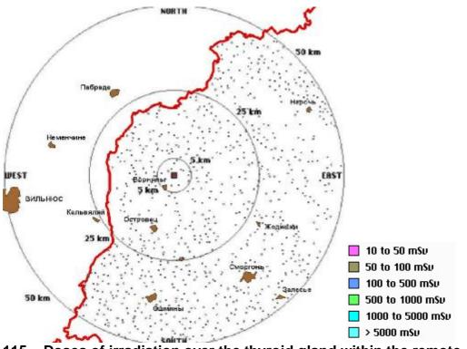
Figure 115 – Doses of irradiation over the thyroid gland within the remote area around NPP under «winter» scenario of maximum design-basis accidents, mSv (mGy)
