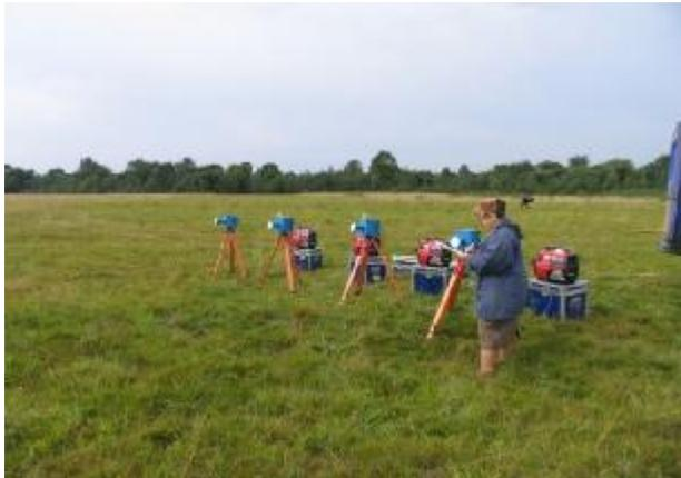
During the field studies made in 2008, atmosphere samples for detection of radioactive aerosol were taken using mobile filter units.
