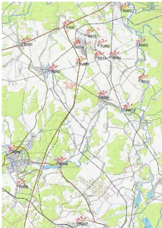
Figure 8.35 Diagram of directions of horizontal motions of points between epochs, 2012-2024
